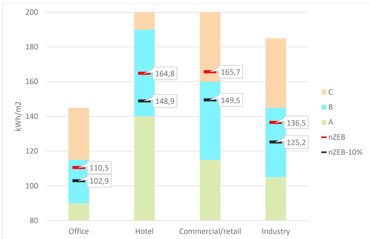
Figure 9 Energy performance with reference to the national definition of NZEB and NZEB-10% compared to limit values in the EPC system
