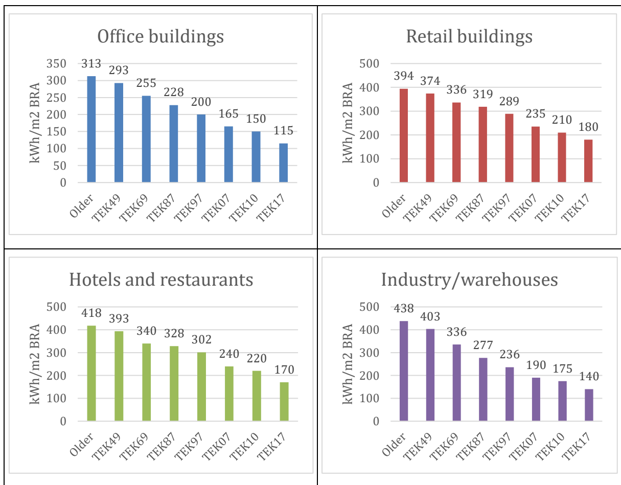
Figure 15 Development in calculated specific net energy demand based on building code and building tradition, (Multiconsult, simulated in SIMIEN)
